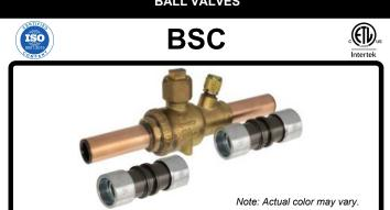
The ball valve assembly provides equal pipe size for the inlet and outlet. Both sides are ready for TUFFLOK couplers. Different inserts are required for soft or hard copper tubing. If you need additional different types of inserts, you can order them separately.
